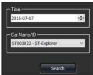
After Selecting “Route” at the top (Fig.4) you will be presented with a larger scale map. At the bottom left corner you will see a window like the one to the left. Here is where you choose the particular day (as far back as 15 days) and the vehicle you want to draw a route for. The device can either be online or offline. Select Search to start the search for all routes for that day.
